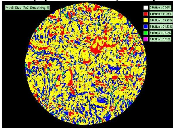
**Fig. 1. The color coding of 10 sccm H<sub>2</sub> flow rate sample in  $7.5 \mu\text{m}$  FOV. The dominant yellow color resembles a bi-layer graphene with the coverage up to  $\sim 60\%$  of total area.**
