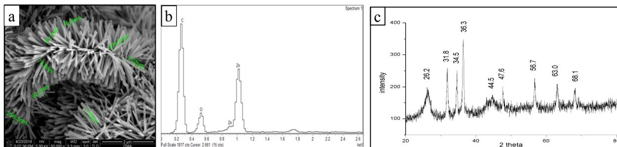
**Fig. 1 (a): FESEM image of CNTCZnO hybrid, (b) EDX analysis of CNTCZnO and c) XRD pattern of CNTCZnO**
